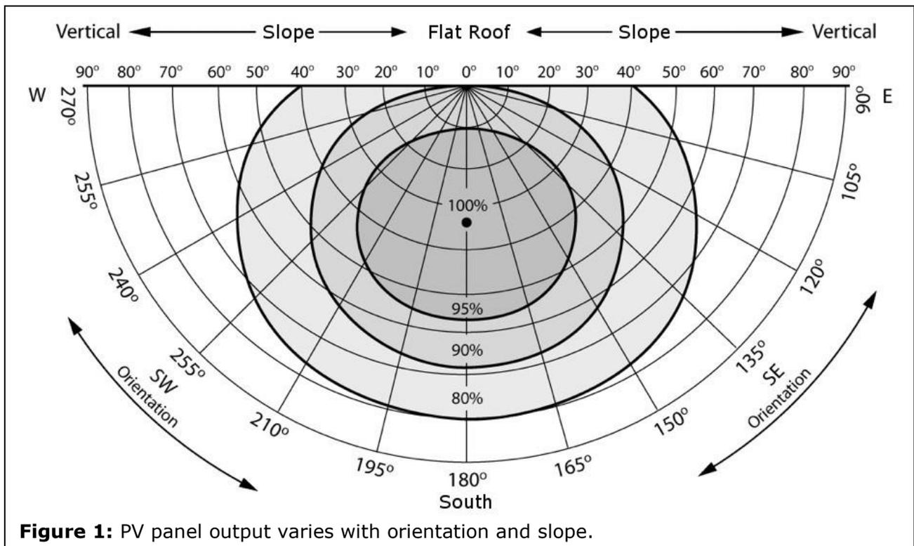
**Figure 1:** PV panel output varies with orientation and slope.
